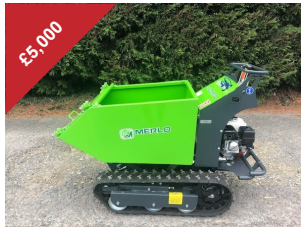
MERLO CINGO M500 Handle material in small spaces/steep ground Width 690 mm wide.
